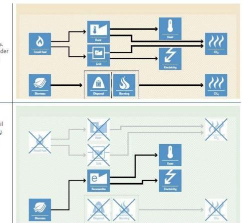
The proposed project activity uses bagasse as fuel for cogeneration unit. The bagasse being a renewable bio- mass fuel does not add any net carbon-dioxide to the atmosphere because of the carbon recycling during growth of sugar cane. Therefore, the project activity will lead to zero CO2 on-site emissions associated with bagasse combustion.
